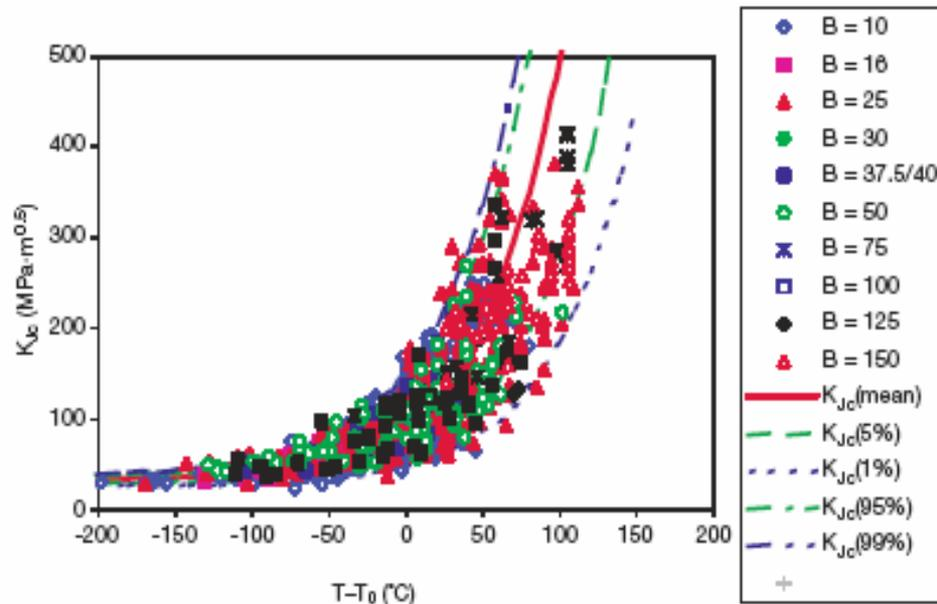
FIG. 17. Temperature dependence of static fracture toughness data for WWER-440 RPV materials.
