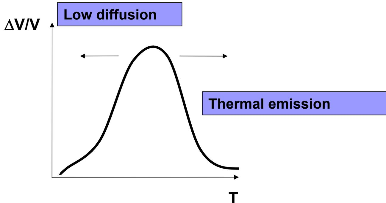
Most metals swell in temperature range of  $0.3 T_m < T < 0.55 T_m$
