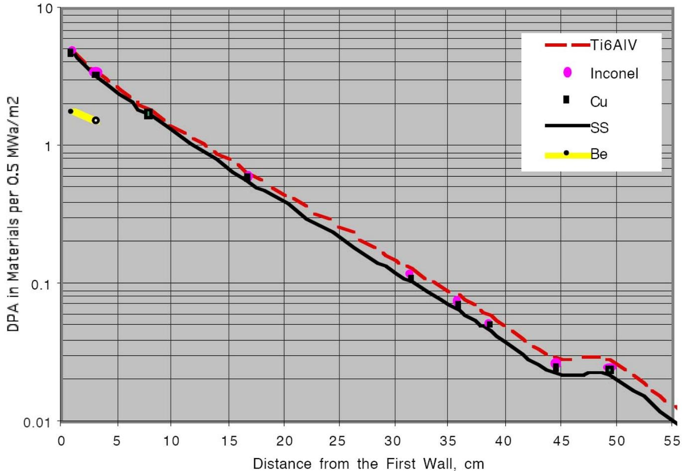
Radial dpa distributions in the bulk shielding blanket for different materials
