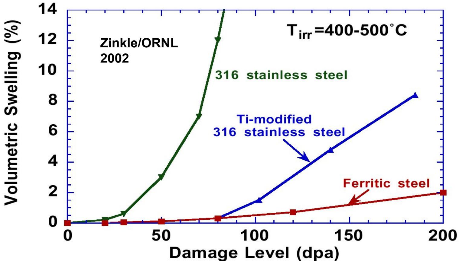
Lowest swelling is observed in body-centered cubic alloys (ferritic steel)
