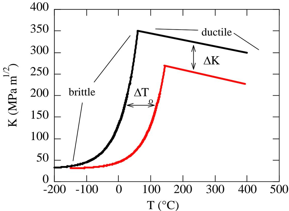
Like other bcc metals and alloys, "ferritic" steels exhibit a ductile-brittle transition of their fracture mode.
