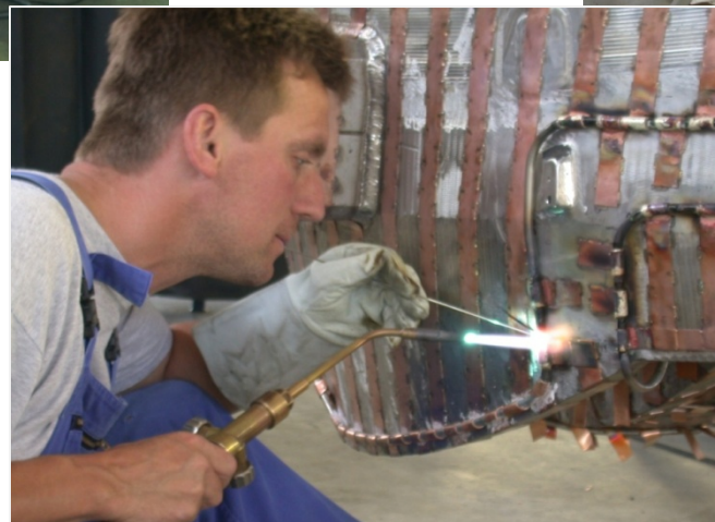
Soldering of Cu stripes to the SS cooling tube
