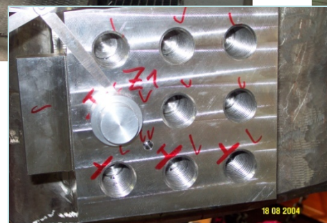
Check of threads with templates
