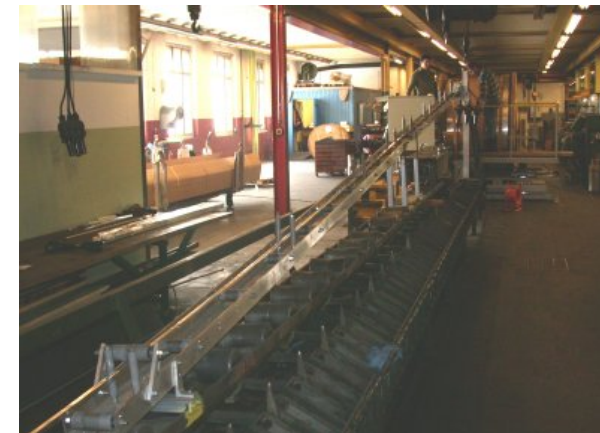
Quenching of hot conduit with water
