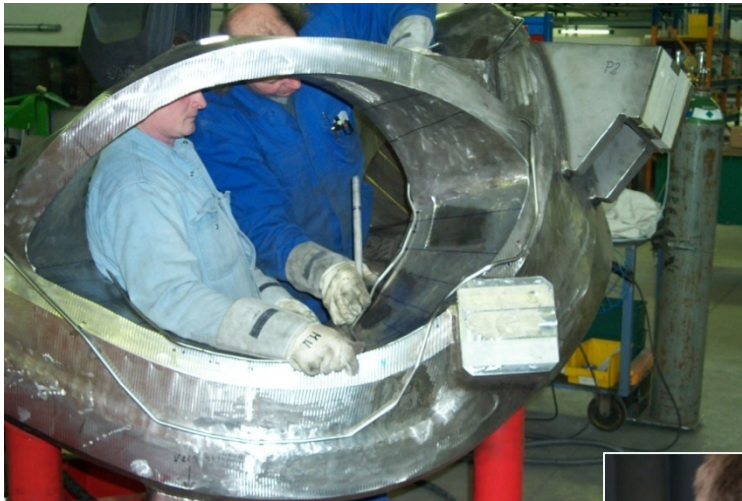
Fitting of the cooling tubes
