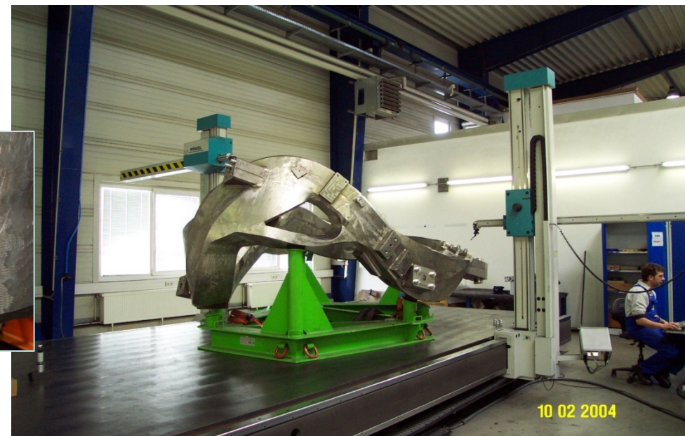
Automatic 3 D measurement of coil after final machining
