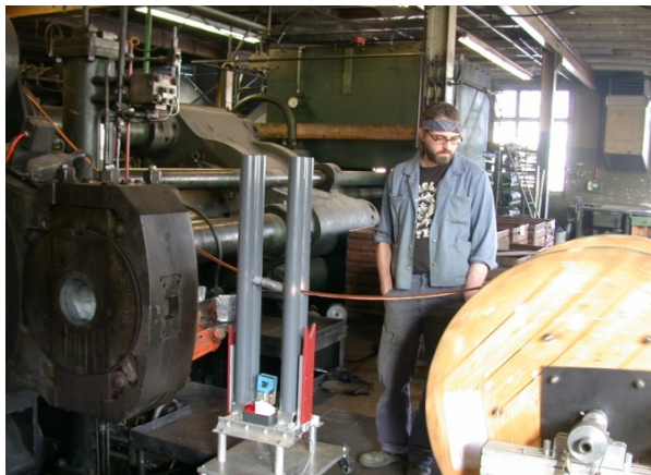
Feeding of rope into press
