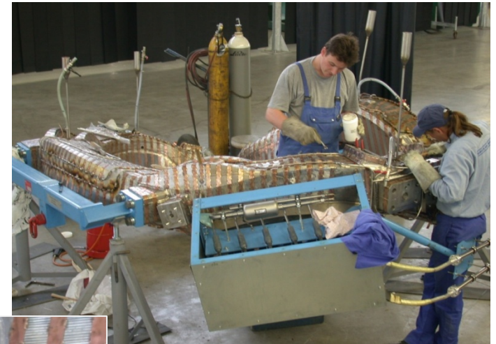
Welding of Cu strips
