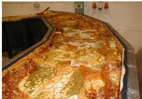
Assembly of impregnation form into impregnation vessel
