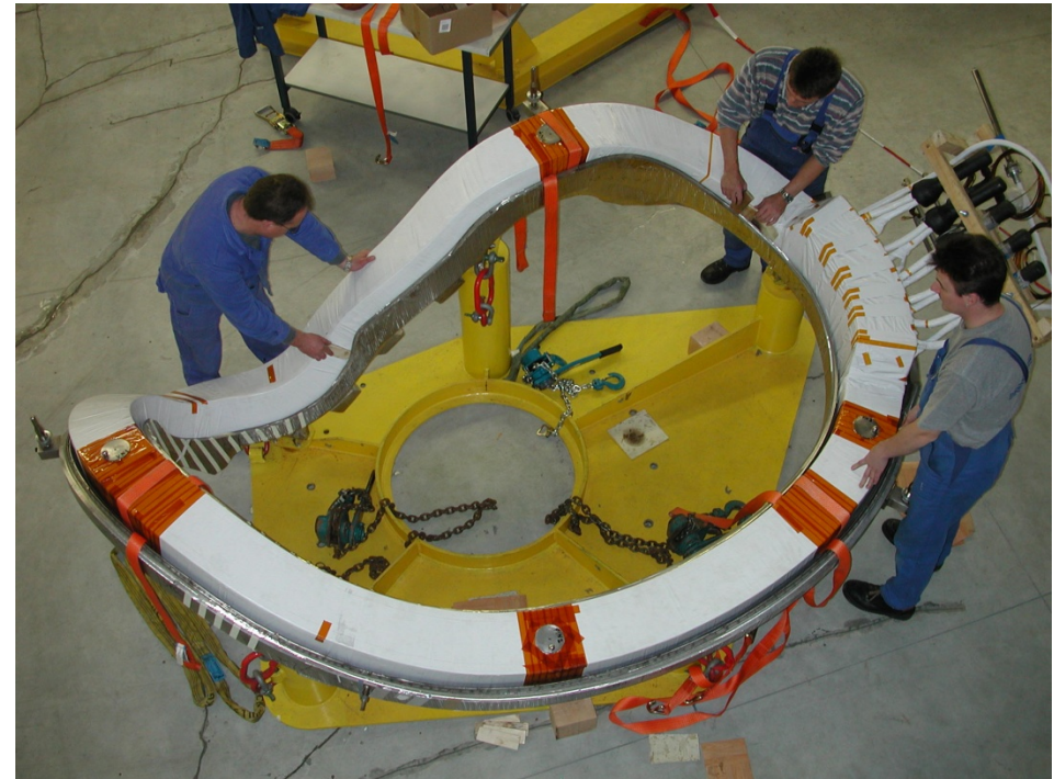
Insertion of winding pack into Case
