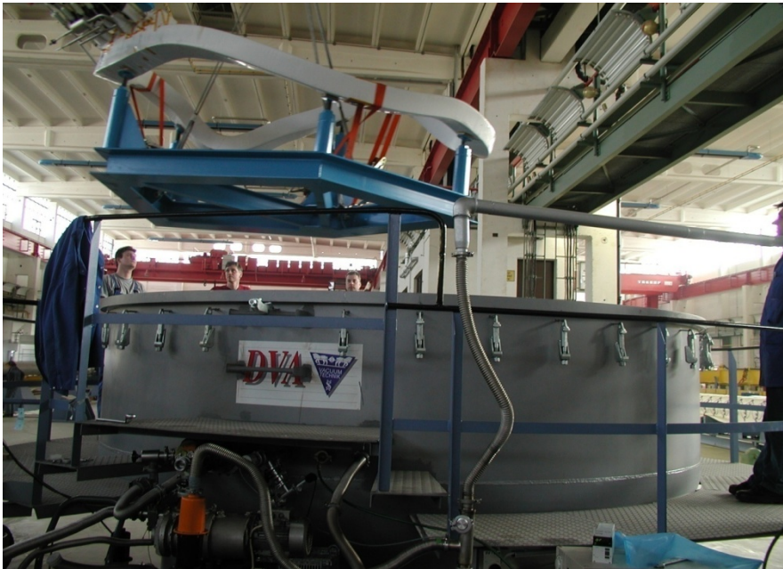
Leak test of Winding Pack
