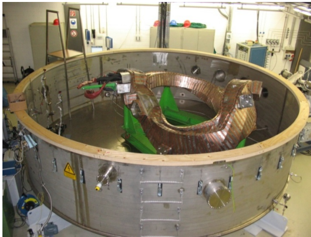
1. High voltage test of the coil in vacuum („Paschentest“ )
