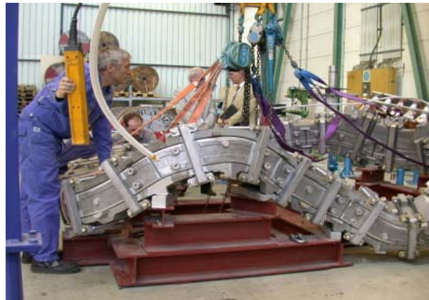
Assembly of winding pack into impregnation form
