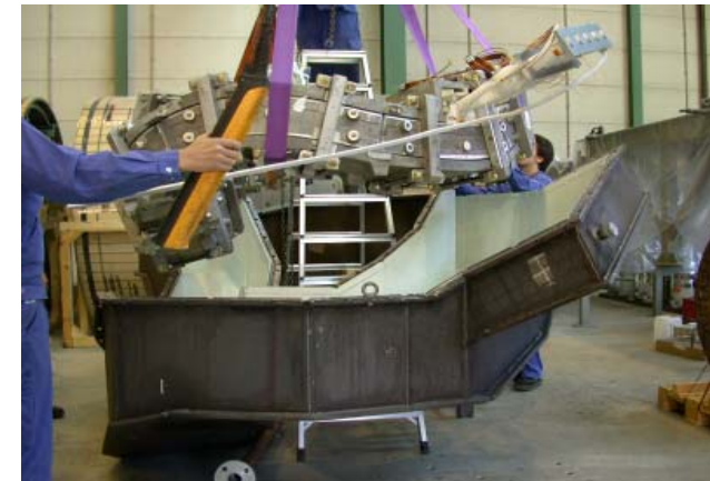
Assembly of impregnation form into impregnation vessel
