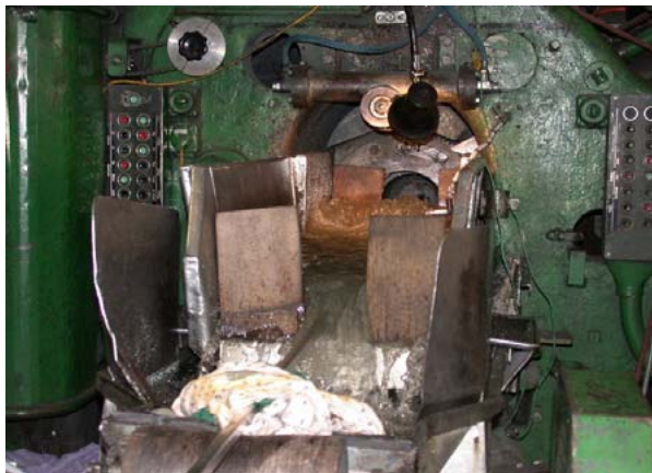
Quenching of hot conduit with water
