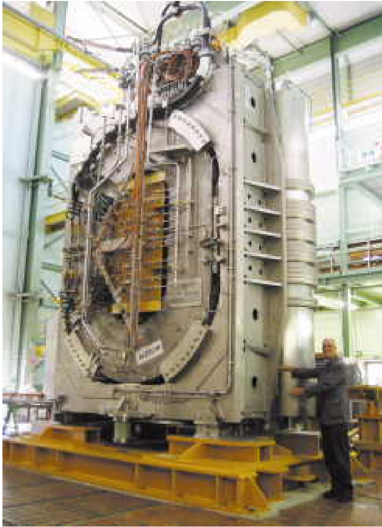
The 112 t test configuration for the test of the TFMC in the background field of the LCT coil
