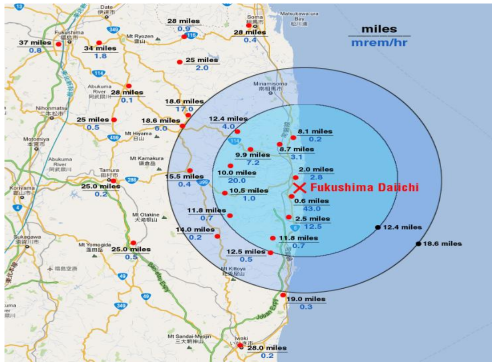
Figure 5.4-1 Initial Off-Site Survey Results
